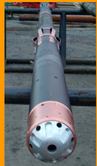
The DIVERTA™ and N-line centraliser ready to go in the hole
